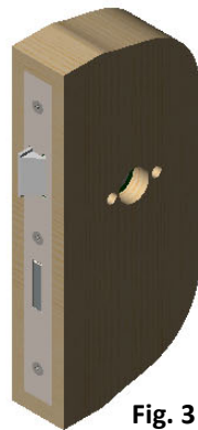
Holes at 38 CRS for BB fixing
