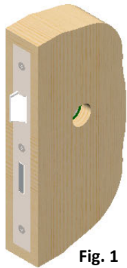
Door prepped with Ø25 hole using lock fitting instructions
