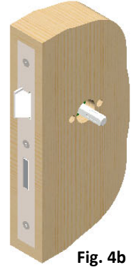
Spindle passed through lock follower leaving equal projection to both sides
